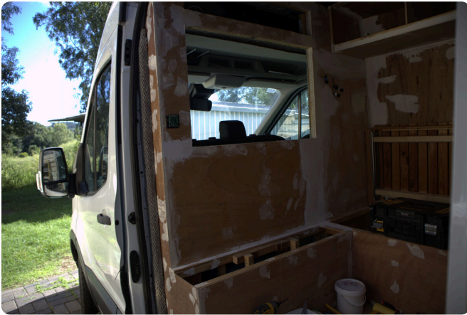
The whole interior filled, sanded and ready for paint
