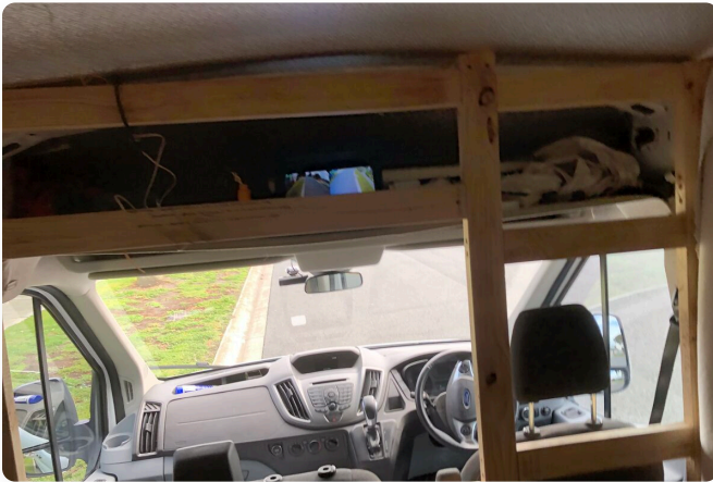
Building the insulated cockpit dividing wall — using reclaimed wood from the original panels
