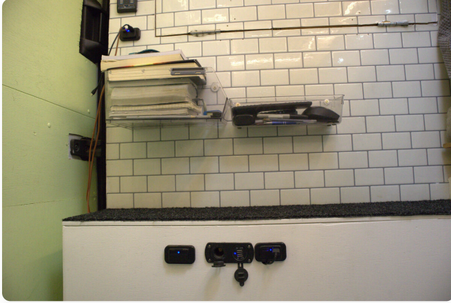
USB charging points throughout the van, and the wiring behind them
