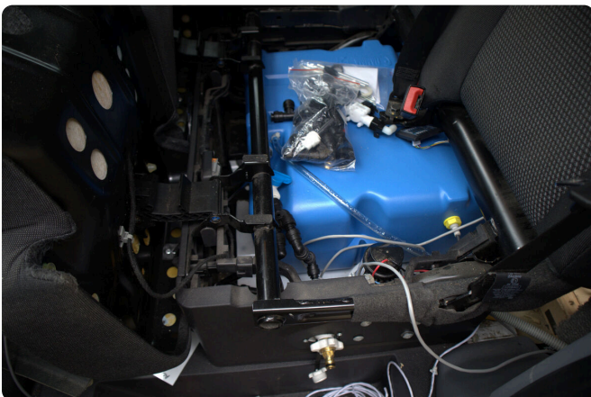
Fresh water tank tucked under the seats with the pump mounted right beside it
