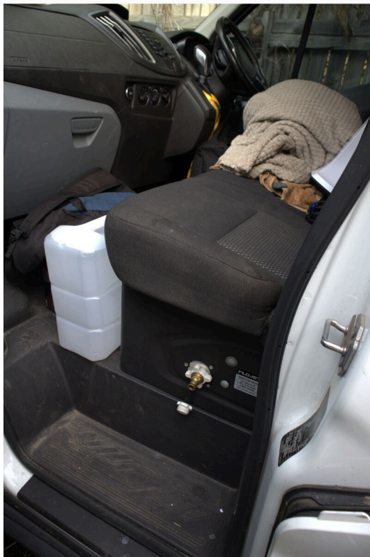
Fresh water inlet — keeping it simple and accessible
