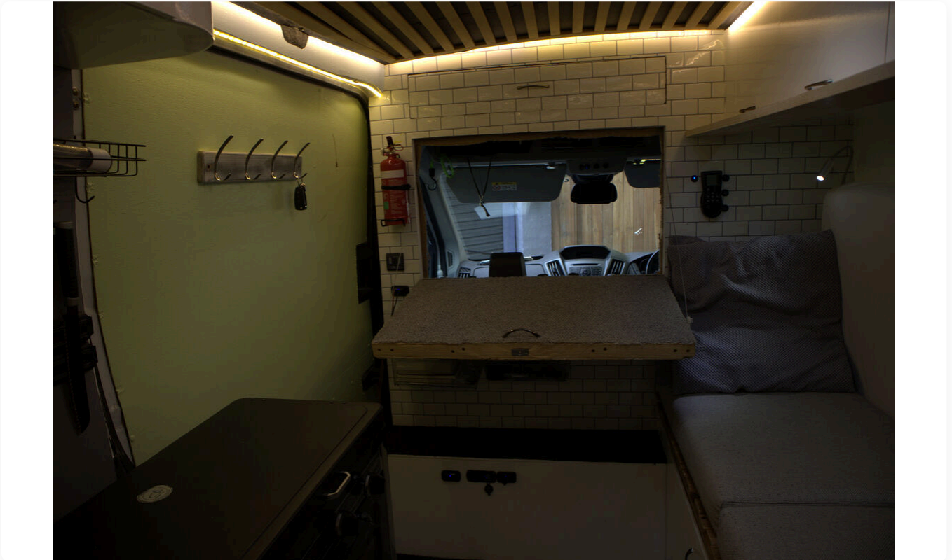
Drop-down shelf accessible from the cockpit — added during upgrades
