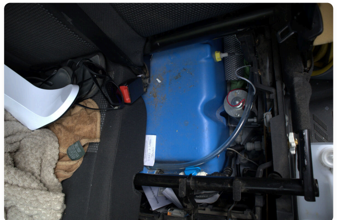
Fresh water tank tucked under the seats with the pump mounted right beside it
