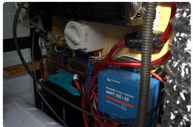
Lithium battery upgrade and solar controller wiring
