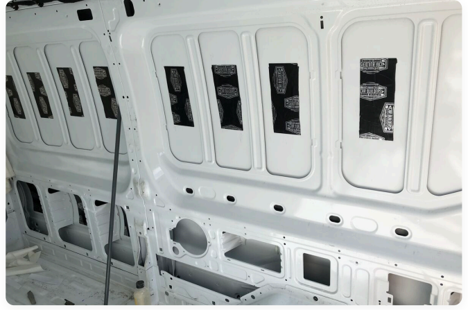
Sound deadening mats applied to every bare metal panel before anything else goes in
